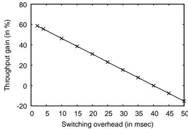
**Figure 13:** Impact of switching overhead on TCP throughput.
