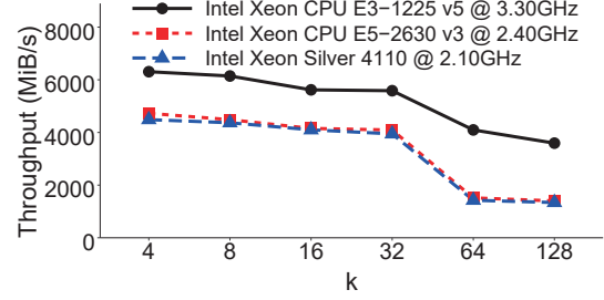
Figure 1: Encoding throughput on different Intel CPU families versus k for a chunk size of 64 MiB and n - k = 4 .
