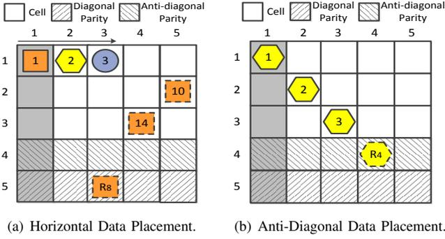
Fig. 6: Explanations of Motivation 1, based on X-Code over  $p = 5$  disks. Anti-diagonal data placement (figure (b)) retrieves fewer elements than horizontal data placement (figure (a)) for the degraded read  $\{\#1, \#2, \#3\}$ . The shape with dashed line denotes the extra element to be read for data recovery.
