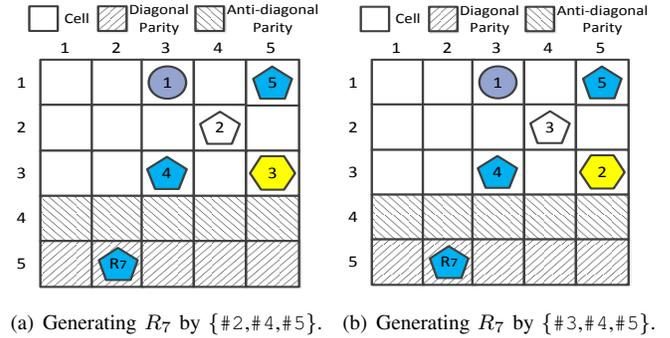
Fig. 11: An example to refine the data placement when generating  $R_7$ . In this example,  $R_{cur} = R_1$  and  $R_{next} = R_7$ , where sequential data elements  $\{\#1, \#2, \#3\}$  is placed to generate  $R_1$ .
