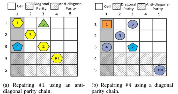
Fig. 8: Explanations of Motivation 3, based on X-Code over  $p = 5$  disks. By switching the positions of  $\#2$  and  $\#3$ , we ensure that sequential data elements are placed in both the anti-diagonal parity chain (figure (a)) and the diagonal parity chain (figure (b)).
