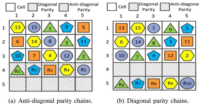
Fig. 12: Data placement of X-Code ( $p = 5$ ) after refinement.
