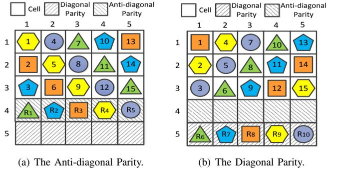
Fig. 4: Element layout of X-Code under vertical data placement over  $p$  disks ( $p = 5$ ).
