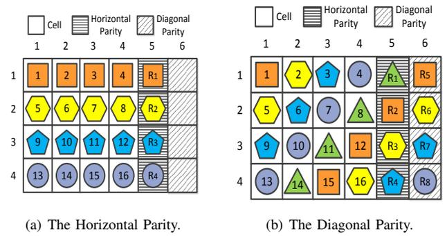
Fig. 1: Element layout of RDP Code under horizontal data placement over  $p + 1$  disks ( $p = 5$ ). Note that the numbers in data elements represent the logical order of how the data elements are stored, and the elements with the same shape belong to the same parity chain for a given encoding direction. We use these representations in our illustrations throughout the paper.
