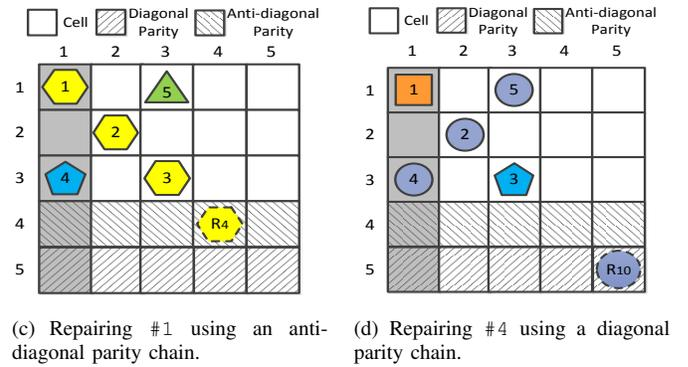
Fig. 7: Explanations of Motivation 2, based on X-Code over  $p = 5$  disks. Anti-diagonal data placement retrieves additional elements from anti-diagonal parity chains (figure (a)), and reads more extra elements when using diagonal parity chains (figure (b)). However, if we place sequential data elements first in an anti-diagonal parity chain (figure (c)) followed by a diagonal parity chain (figure (d)), we can retrieve fewer additional elements.
