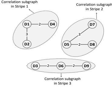
Fig. 5. An example of three correlation subgraphs (suppose  $k = 3$ ). There are three stripes, where  $\mathcal{D}_1 = \{D_1, D_2, D_4\}$ ,  $\mathcal{D}_2 = \{D_5, D_7, D_8\}$ , and  $\mathcal{D}_3 = \{D_3, D_6, D_9\}$ . Then the correlation degrees of the data chunks in the three subgraphs are  $R(\mathcal{D}_1) = 5$ ,  $R(\mathcal{D}_2) = 5$ , and  $R(\mathcal{D}_3) = 4$ , respectively.
