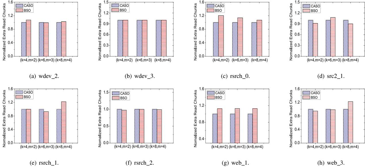
Fig. 11. Experiment 4 (Normalized ratio of additional data read in degraded reads.) Smaller values indicate less data are retrieved in degraded reads.
