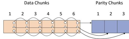
Fig. 1. Encoding of the  $(6, 3)$  RS code for a stripe, in which there are six data chunks and three parity chunks. If one of the data or parity chunks is lost, any six surviving chunks within the stripe can be used to reconstruct the lost chunk.
